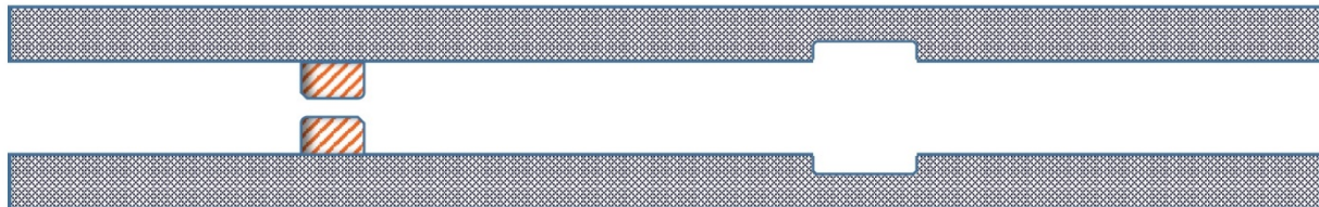
Figure 1: Schematic description of typical blockage and ID wall loss in a tube
